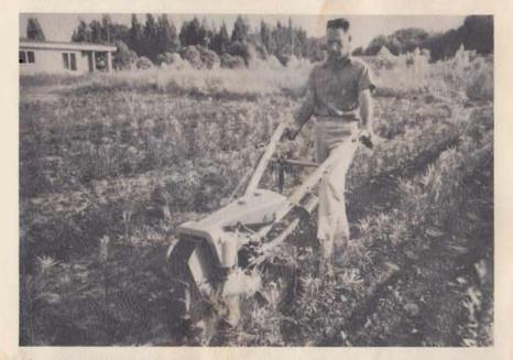
The GRAVELY Model D gives a total Tractor width of only 15 inches at the widest part. It cultivates any row a man can walk through. You have a clear view of the front mounted tools. You can always see just where they are working. The tools are on an adjustable Tool-holder, to handle any width of row.
